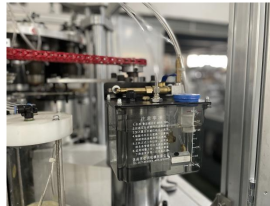
METHYL SILICONE OIL WASTE OIL TANK) 2
